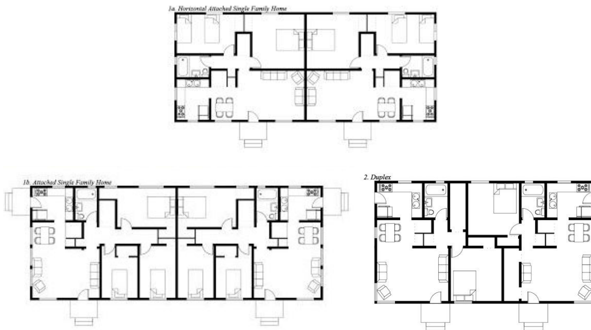
Figure 9. Single Family Attached Duplex Unit Floor Plans. Linda Vista Defense Housing Plans. Beckman, Donald S. Cameron and Gerard. "Linda Vista America's Largest Defense Housing Project."
