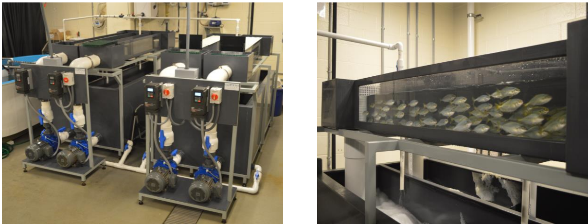
Figs. 2, 3: Two views of custom raceways designed to exercise the fish at optimal swimming speeds
