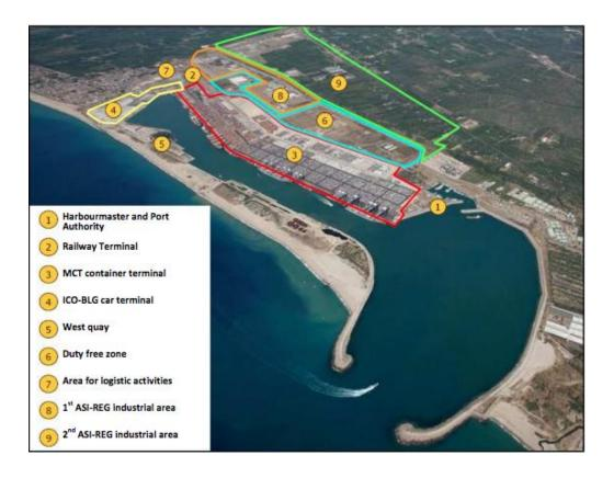
The square strips of color above the channel (highlighted in red) are container loading and temporary storage areas, officially called the Medcenter Container Terminal. Above the large container terminal are vacant industrial areas. The administrative center containing the offices of the Harbormaster, Port Authority, and Port Security are located in Zone 1.
