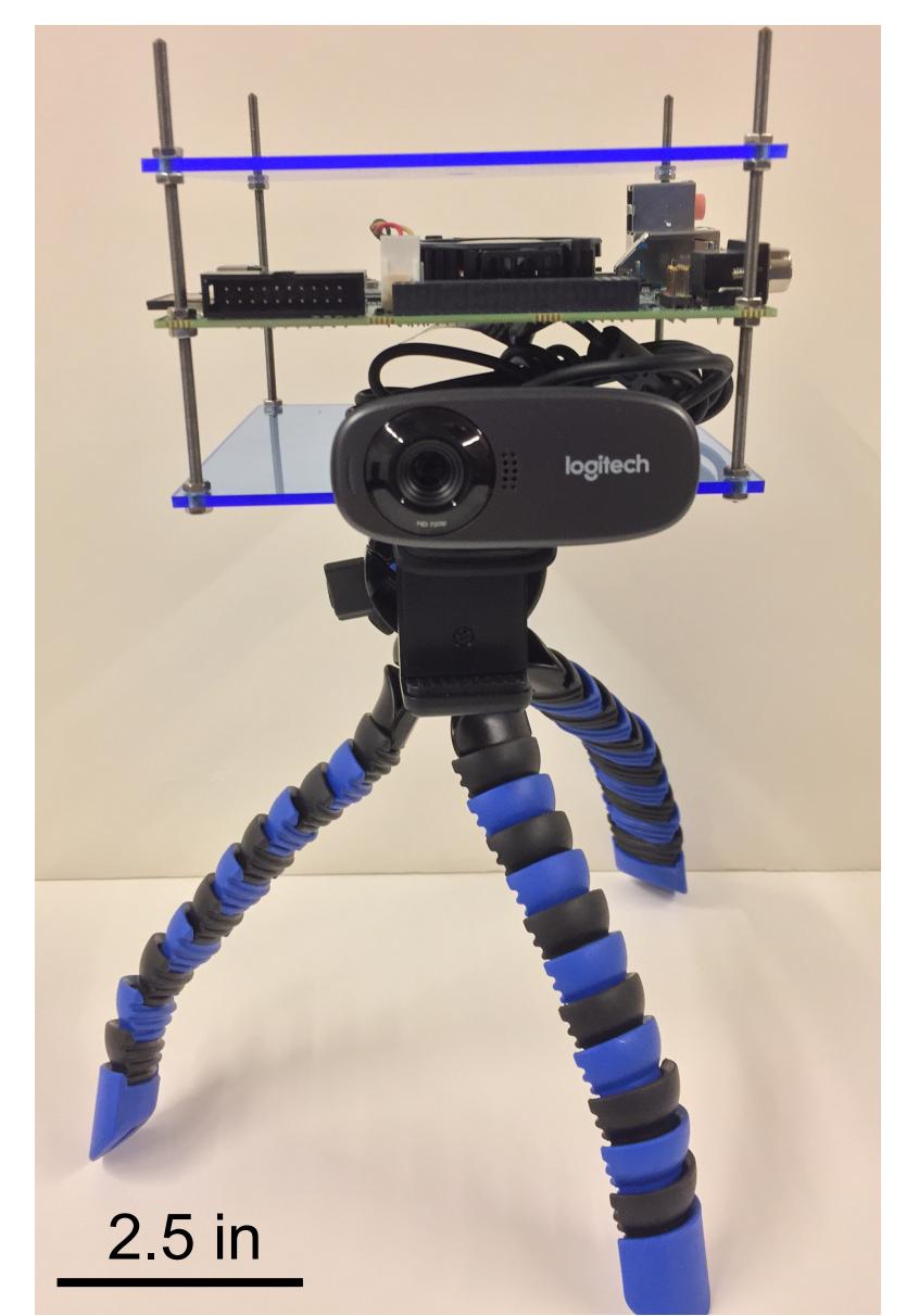
Figure 3. Standing fume hood monitor setup
