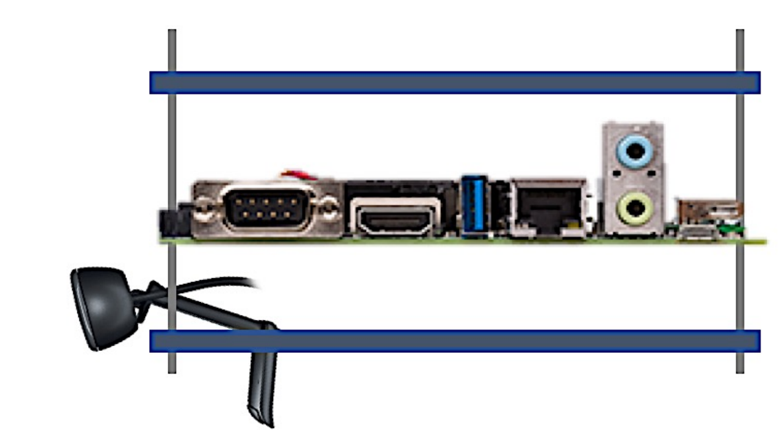
Figure 5. Fume hood monitor side view, with detail of ports on TK1 and profile of the camera
