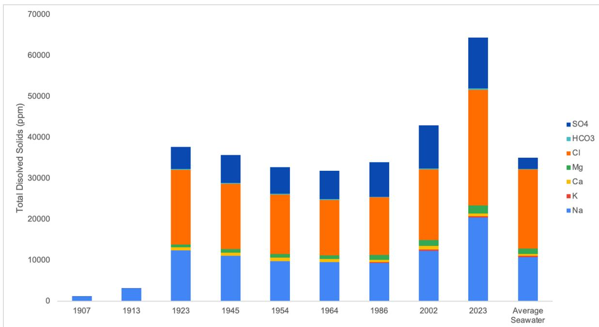
Figure 5. Total dissolved solids (mg/L) compared over time and to average seawater. The 2023 data comes from the current study while all previous years come from Holdren & Montañó (2002), Cory, (1915), Hely, (1966), and Setmire, (1990).
