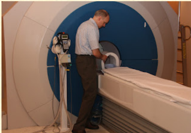
Dr. Hoby Hetherington places a special head detector in the 7 Tesla MRI scanner in his lab at Yale University (photo by Gene Veritas).
