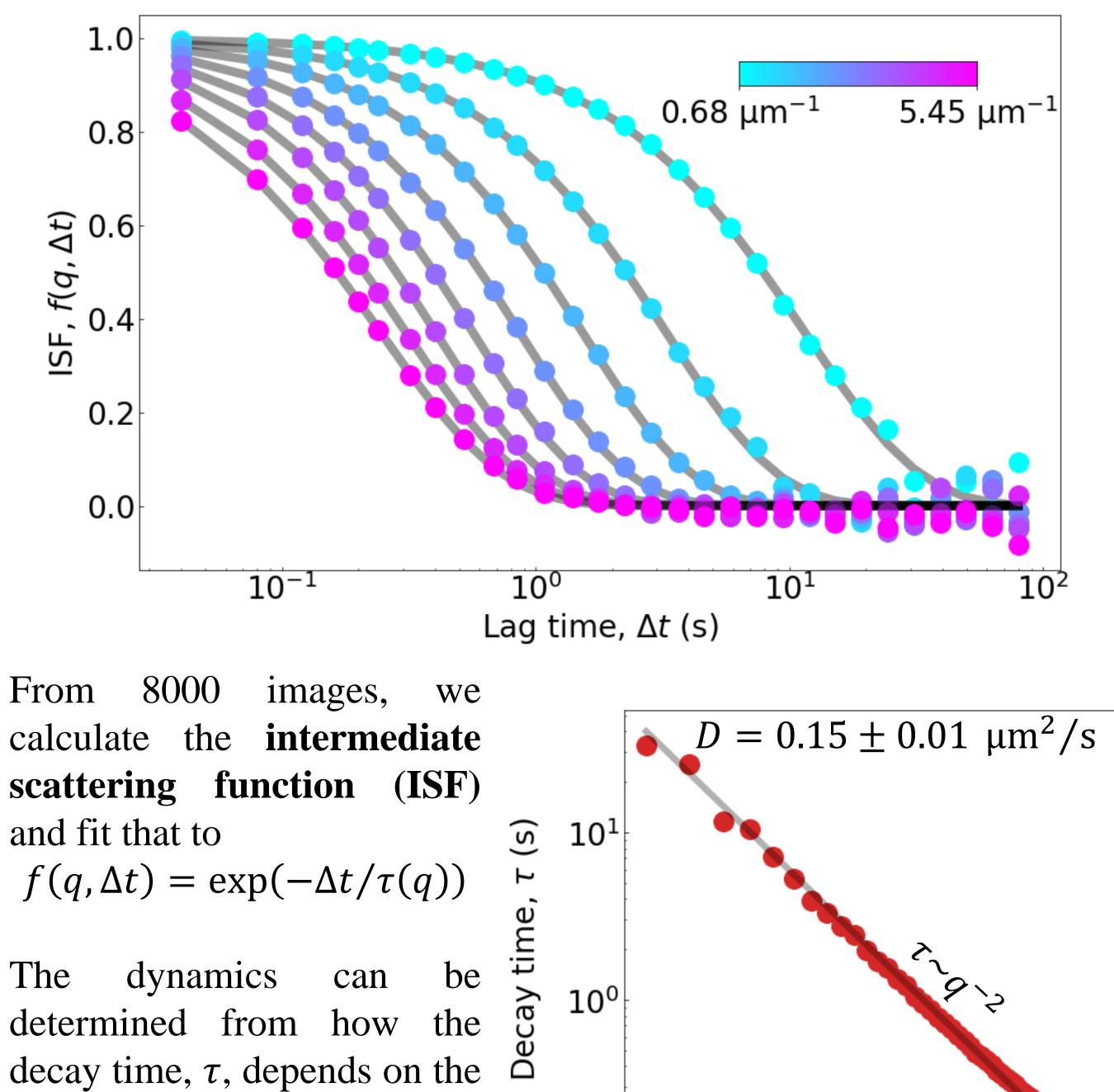
From calculate the **intermediate** scattering function (ISF) and fit that to
