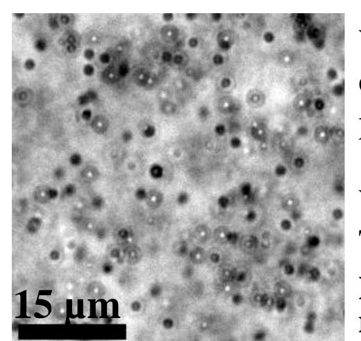
With DDM, we determine the **diffusion** coefficient micron-sized of particles in solution.
