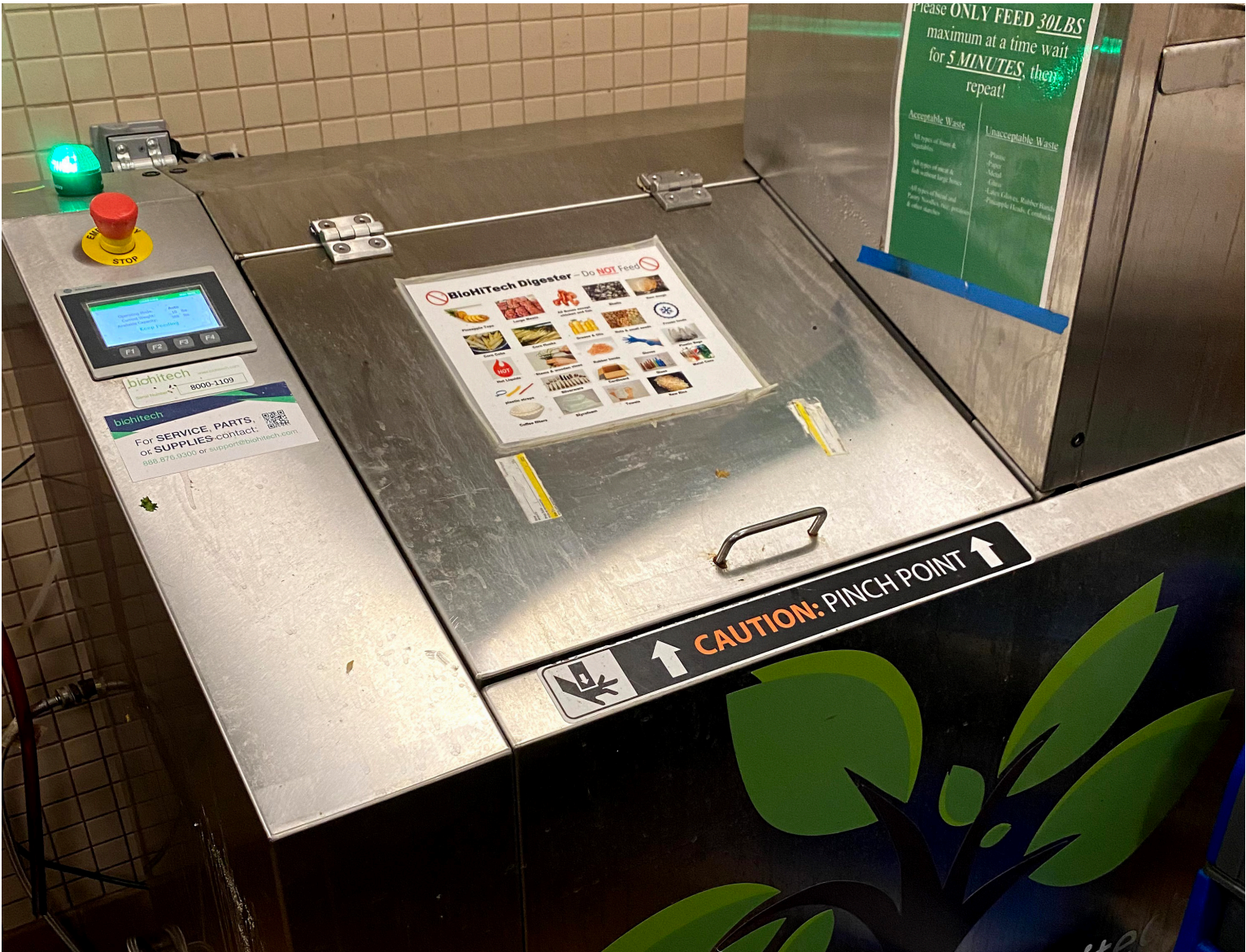
The BioHiTech Digester is a tool that utilizes food waste and repurposes it to be broken down into waste water.
