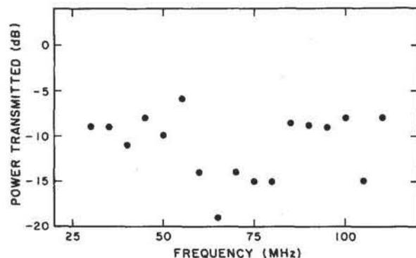
FIG. 2. Lower-hybrid wave power transmitted through grid, compared to wave power approaching grid, versus wave frequency.
